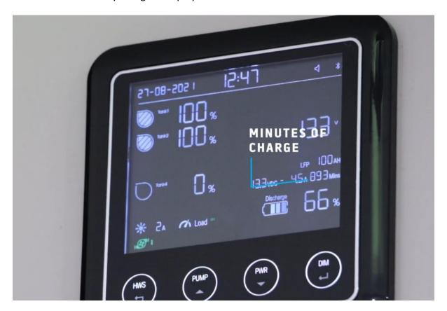
As displayed on the screen, this RV has 893 minutes of solar charge/battery capacity.
